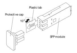
Figure 75. Unlocking the SFP module latch - plastic variety
